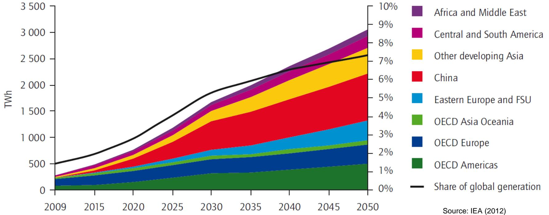
In 2050, IEA estimates 2 460 TWh of electricity will be produced from biomass and waste, a fivefold increase on 2010
