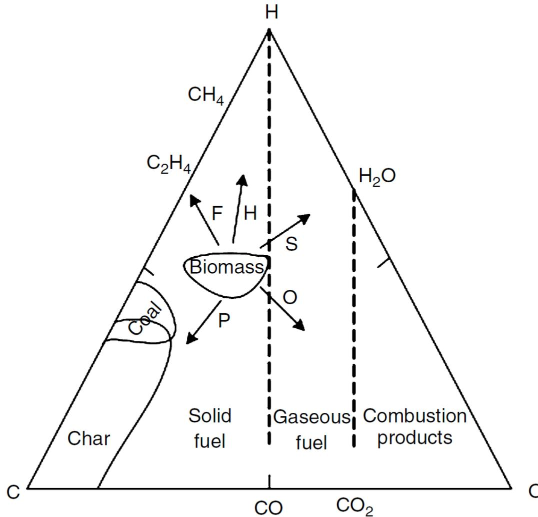
H hydrogen S steam O oxygen P slow pyrolysis
